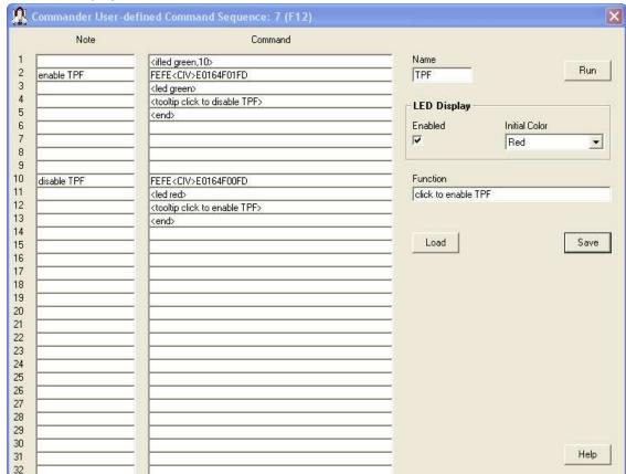
Using LED color to display the state of a controlled element, in this case an Icom IC-7700's Twin Peak Filter:
