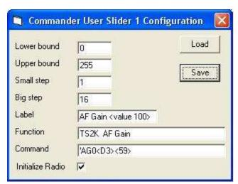
The <D3> substitution command does not specify a Slider number, so Slider 1's value is used (because this is Slider 1's configuration)
